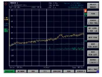
Green trace: R&S<sup>®</sup>FSU-B24 preamplifier and noise correction.
