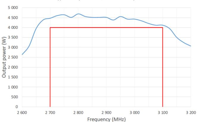
Typical Output Power (Psat @ 0 dBm input)
