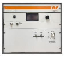
A front panel display indicates the operational status and fault conditions. All amplifier control functions, and status indications are available remotely using GPIB/IEEE-488, RS-232, fiber-optic serial, USB, or Ethernet. Interface connectors are located on the back panel. Local and remote operation is managed by a switch on the front panel.
