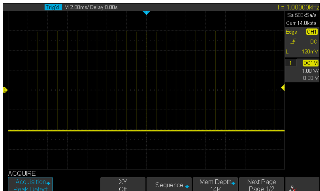
Figure 20 Pulse With 0.1% Duty, Peak Detect Mode
