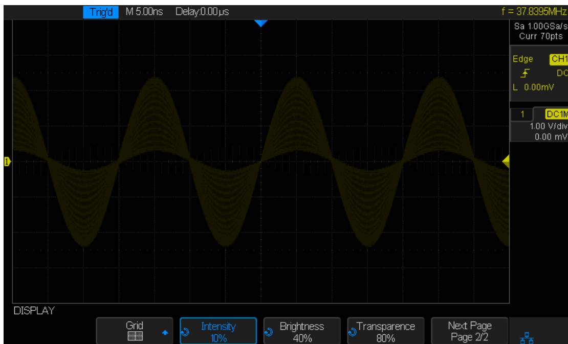
Figure 86: Intensity Set to 10%
