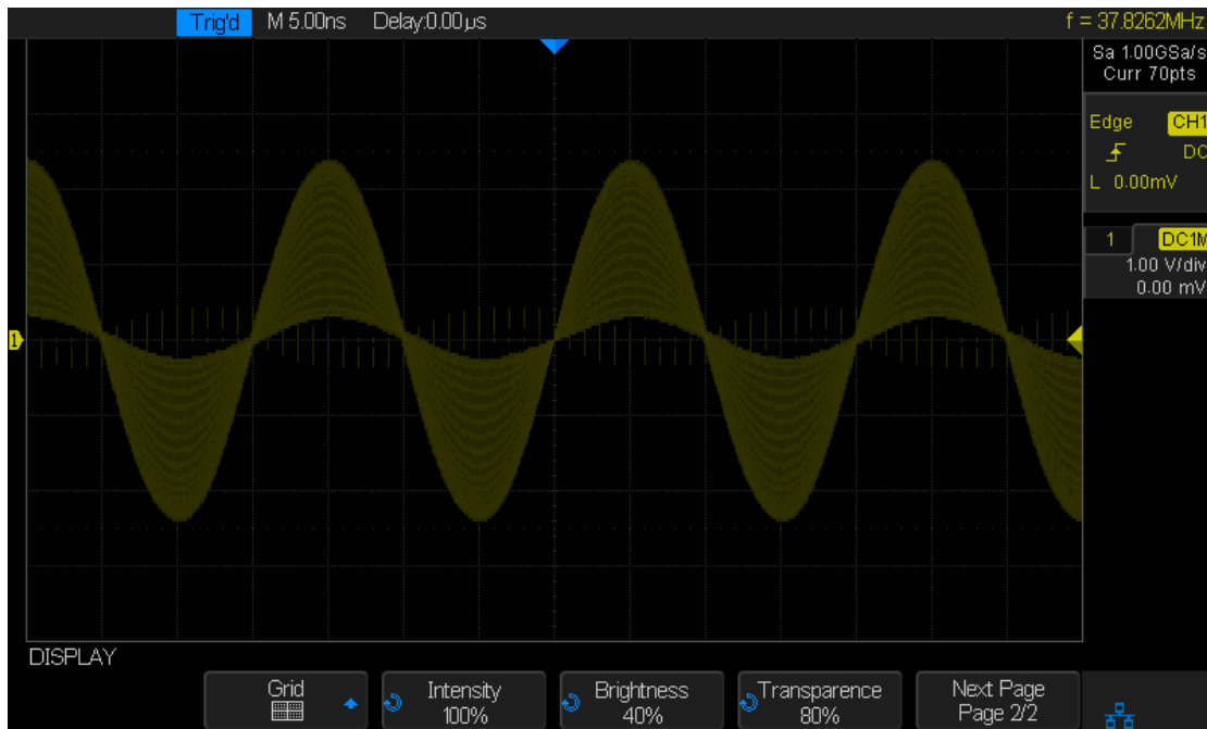
Figure 85: Intensity Set to 100%
