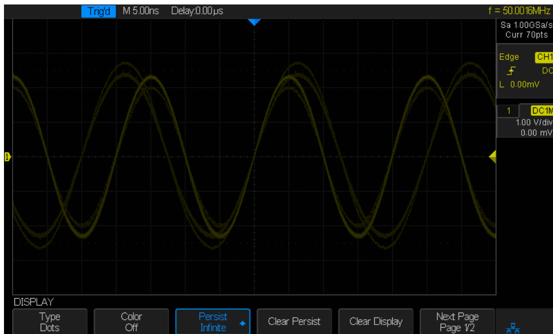
Figure 84: Persist Set to Infinite
