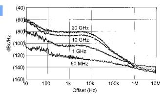
Typical single-sideband phase noise at 50 MHz, 1 GHz, 10 GHz and 20 GHz, 25° C, CW mode. Offsets less than 100 Hz require the high-stability timebase, Option 1F5
