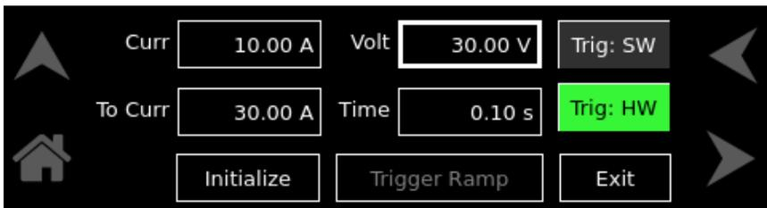
**Figure 3-27. Current Ramp-Screen (HW Trigger)**
