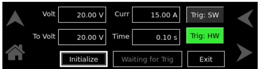
**Figure 3-23. Voltage Ramp-Screen (HW Trigger)**
