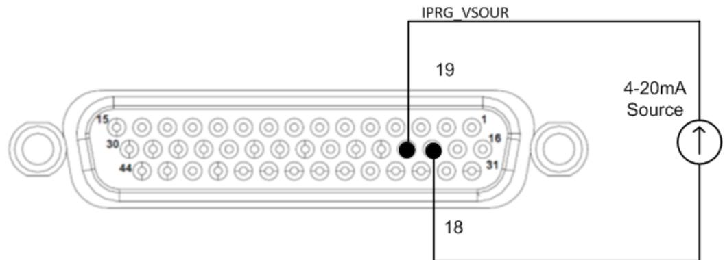
Figure 3-100. Remote Current Programming Using 4-20mA Source
