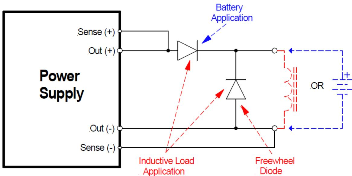
Figure 2-9. Diode Connections
