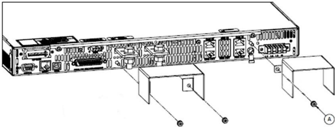
**Figure 2-4. Rear Panel Protective Cover Installation**
