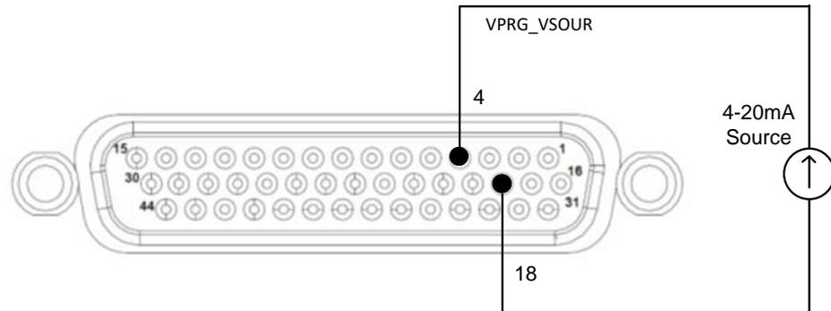
**Figure 3-103. Remote Voltage Programming Using 4-20mA Source**
