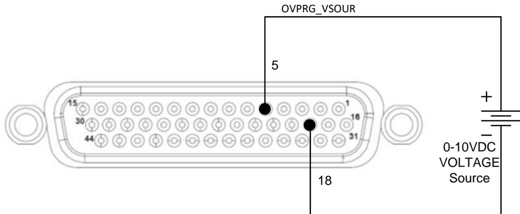
**Figure 3-107. Remote Overvoltage Programming Using DC Voltage Source**
