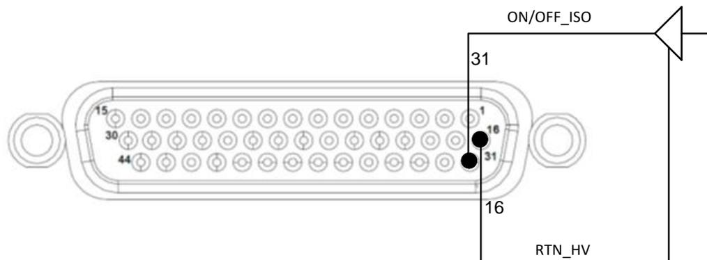
Figure 3-110. Remote Output On/Off Using Isolated TTL/CMOS Source
