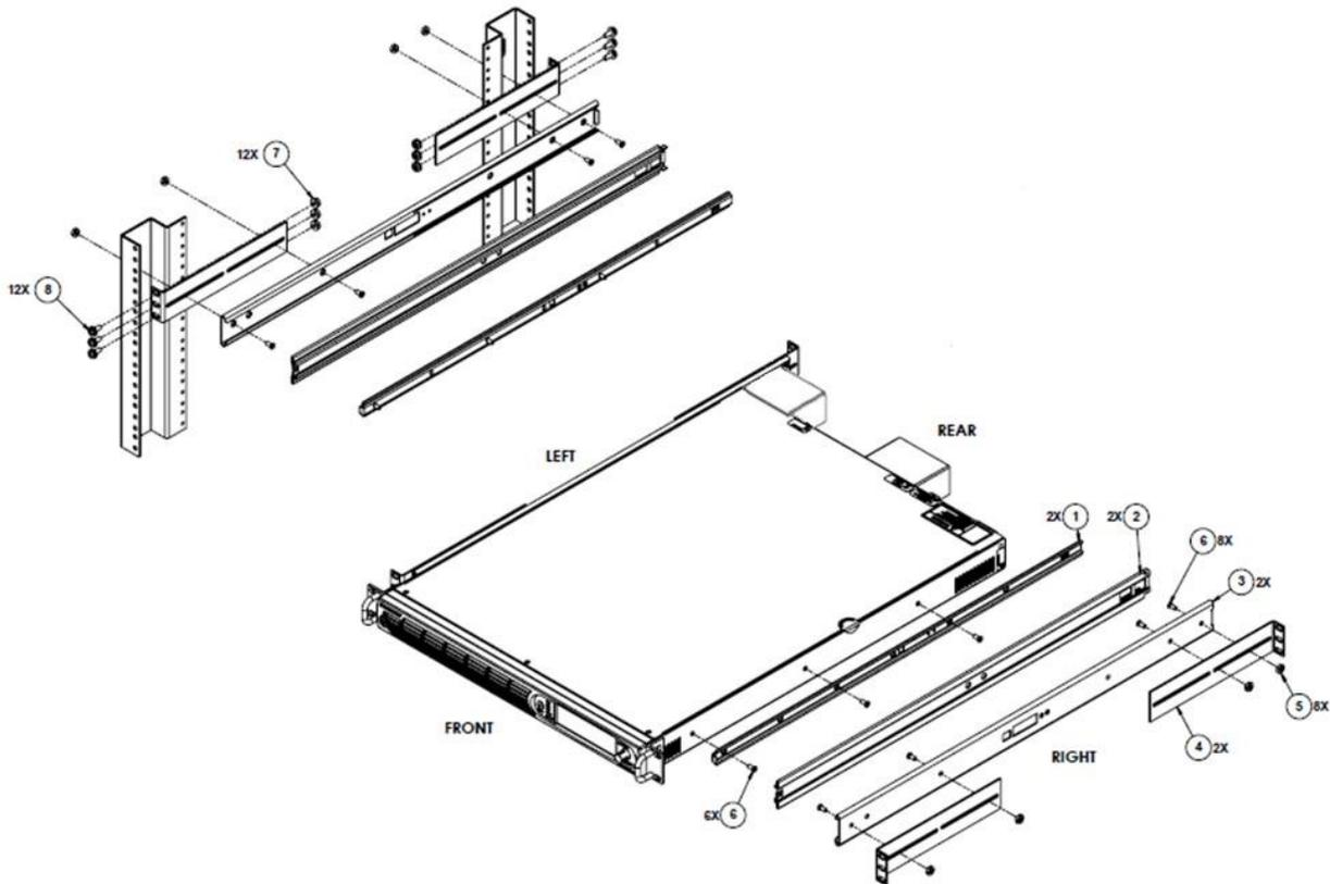
**Figure 2-1. Rack mounting, 1U Models**
