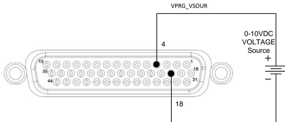
**Figure 3-102. Remote Voltage Programming Using 0-10 VDC Source**
