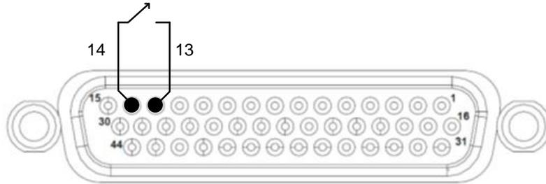
Figure 3-108. Remote Output On/Off Control by Contact Closure
