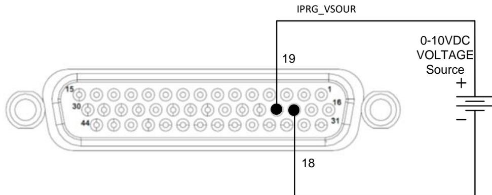
**Figure 3-99. Remote Current Programming Using 0-5 VDC or 0-10 VDC Source**
