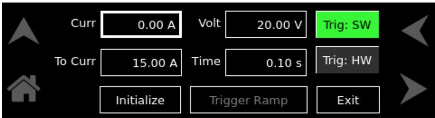
**Figure 3-26. Current Ramp-Screen (SW Trigger)**
