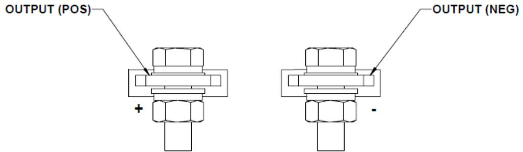
**Figure 2-6. DC Output Busbar**
