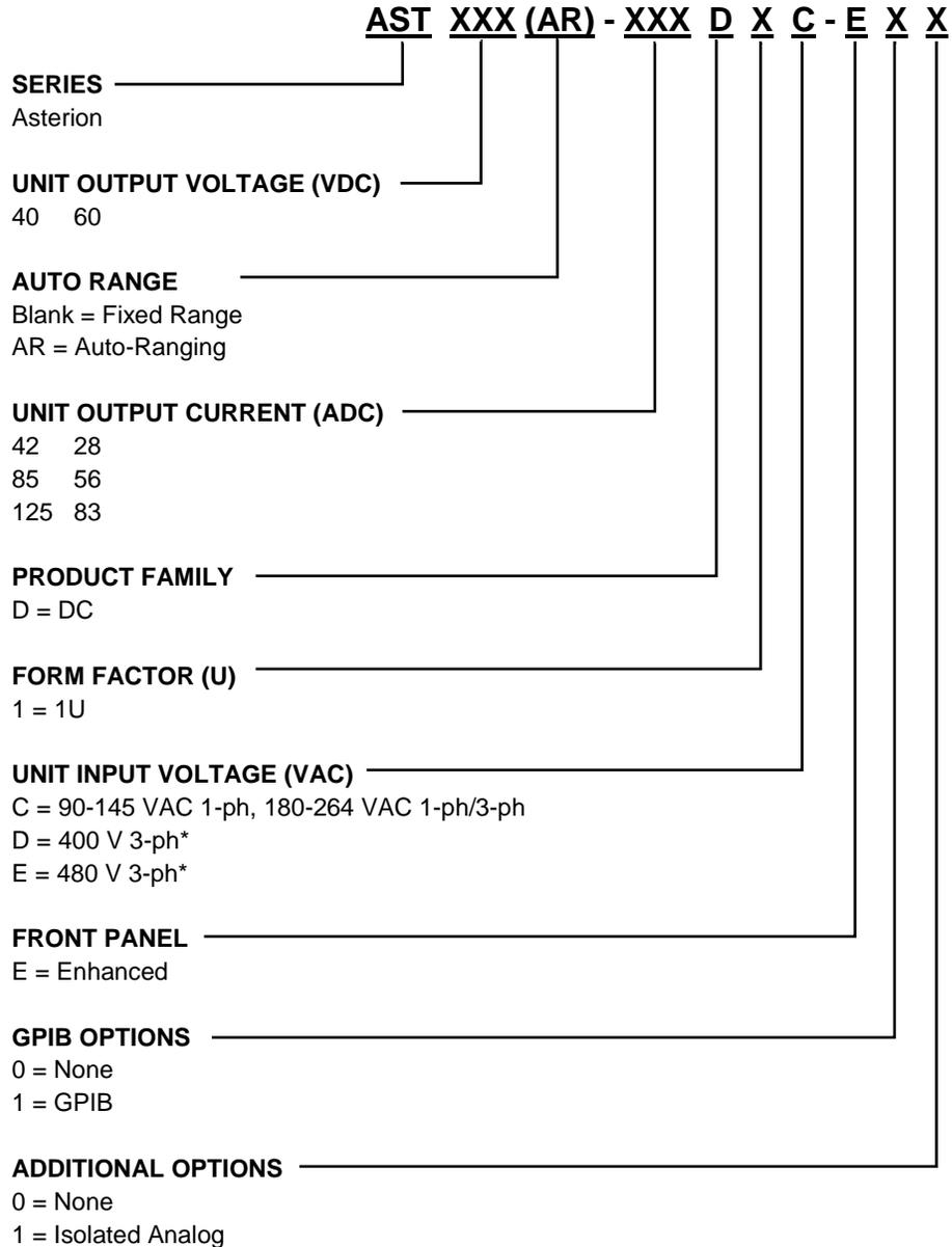
**Figure 1-2. Asterion DC Series Model Number Decoding**
