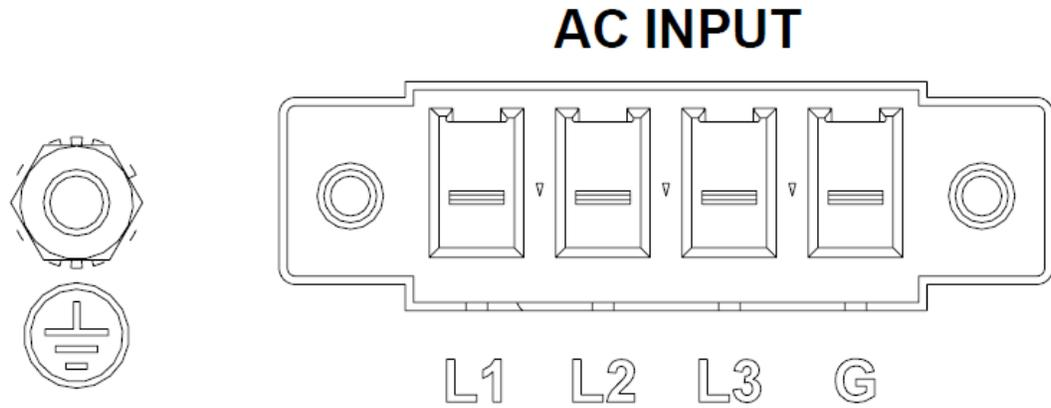
**Figure 2-5. AC Input Connector and Safety-Ground Stud**
