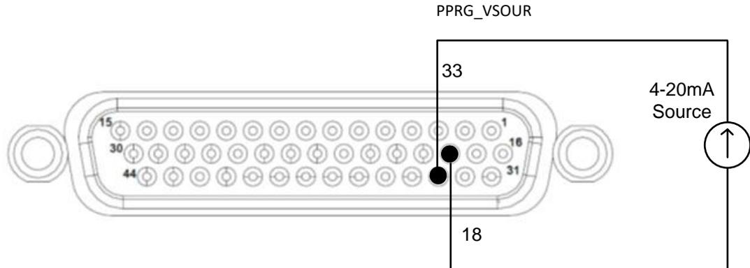
**Figure 3-106. Remote Power Programming Using 4-20mA Source**
