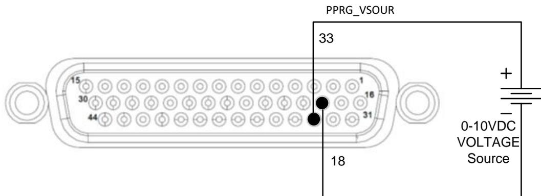
**Figure 3-105. Remote Power Programming Using 0-10 VDC Source**
