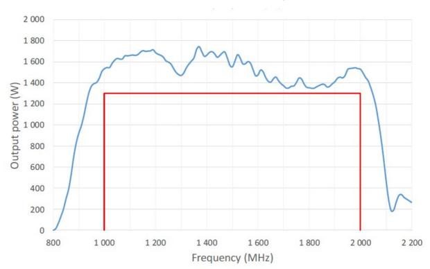
TYPICAL OUTPUT POWER (Psat @ 0 dBm input)
