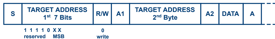
Figure 13-7: 10-bit address, write access
