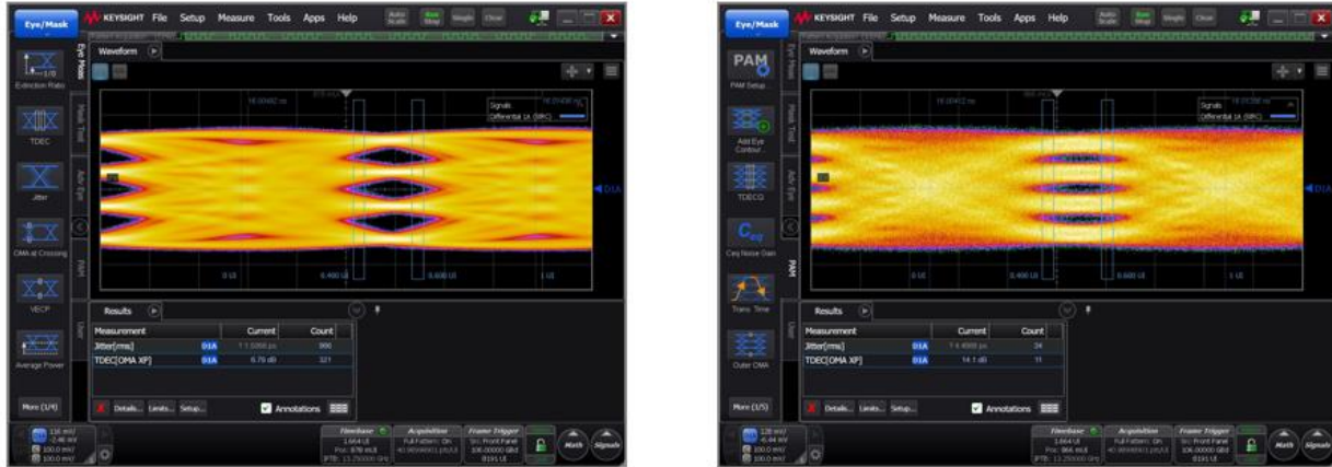
Figure 1. The screens show a 106.25 GBd PAM4 eye diagram without level interference (left) and with random level interference (right) added from M8053A. The example shows a PRBS13Q signal from M8050A high-performance BERT without ISI channel. The s-parameters of the coupler's main path have been de-embedded using the M8070ISIB.
