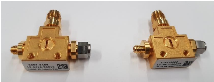
Figure 9. The matched coupler pair M8053A-803 allows injecting the interference signal into a differential data signal before and after the channel to emulate far end and near end injected interference. The matching helps to minimize the skew.
