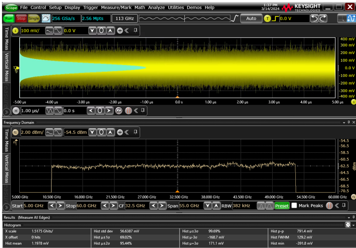
Figure 2. The random interference signal provides a white gaussian noise with up to 64 GHz bandwidth. The upper part of the measurement shows a histogram taken with UXR1104A without attenuator. The lower part of the measurement shows that you can set the minimum and maximum bandwidth of the random interference signal. The spectral noise flatness is excellent within \pm 2 dB.
