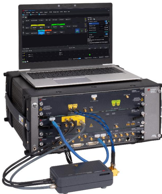
Figure 7. The M8053A interference source can be configured with a M8050A high-performance BERT in one 5-slot AXIe chassis. The M8053A sits in the upper slot. It is also possible to configure the M8053A in a second AXIe chassis. The whole BERT system including the M8053A is controlled by the M8070B system software. This image shows prototype cables and coupler.
