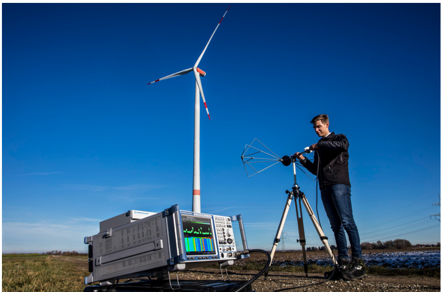
Battery-operated in-situ measurements with the R&S®ESR.
