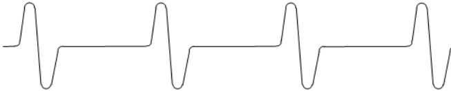
Figure 9. Incorrect Signal Polarity for VR Input Circuit
