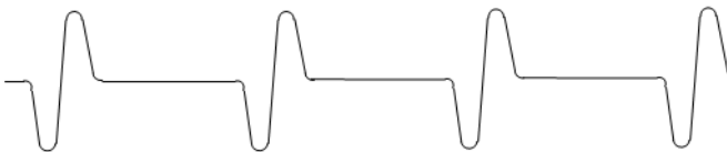
Figure 9. Incorrect Signal Polarity for VR Input Circuit
