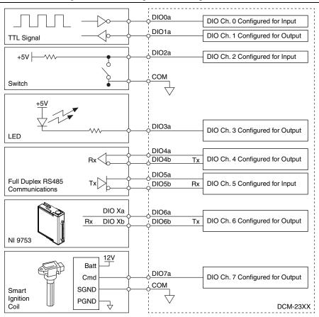
Figure 12. Connecting to External Digital IO Devices
