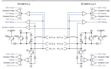
Figure 6. DI Half-H Driver Circuit Topology
