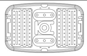
Figure 2. DCM Connector 1 Pinout
