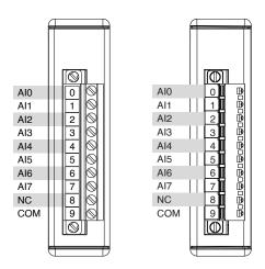
Each channel has an AI terminal to which you can connect a current signal. The NI-9203 also has a common terminal, COM, that is internally connected to the isolated ground reference of the module.
