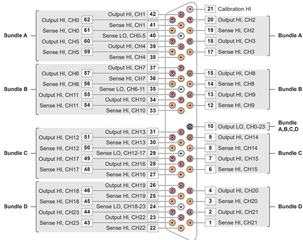
Figure 3. PXle-4163 Pinout with ACC-4163-1
