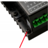
Figure 6. Grounding Screw on the Chassis
