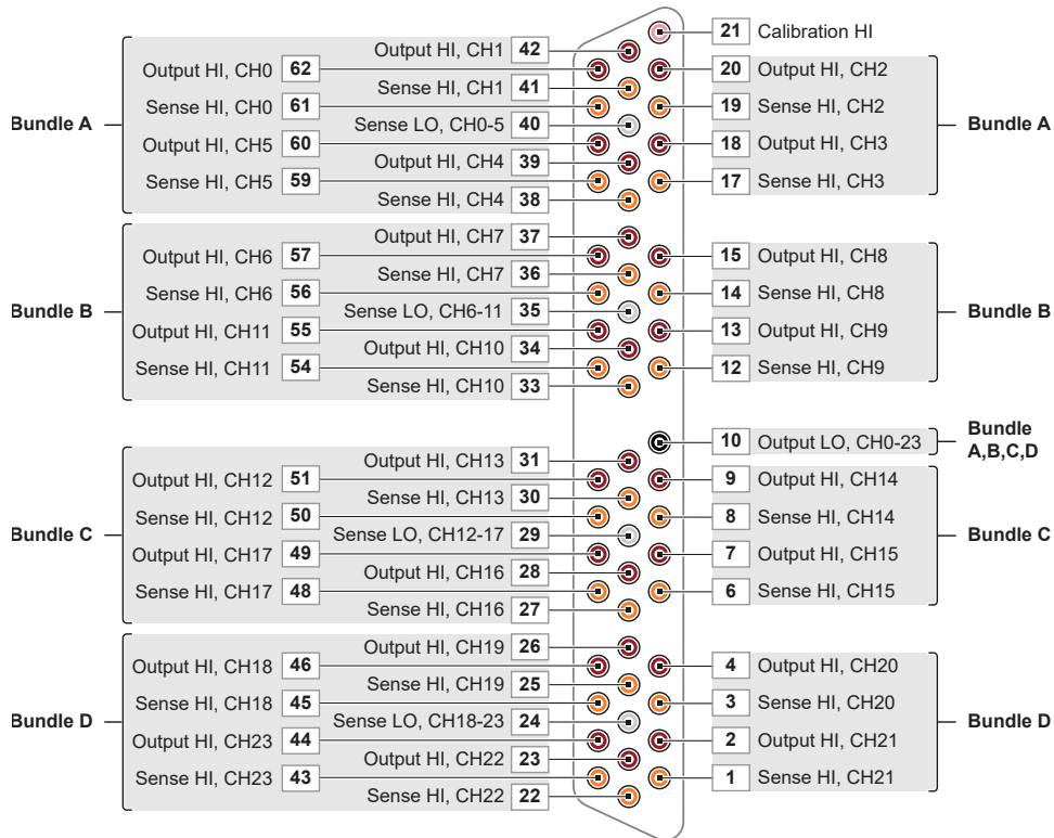
Figure 1. PXIe-4163 Pinout
