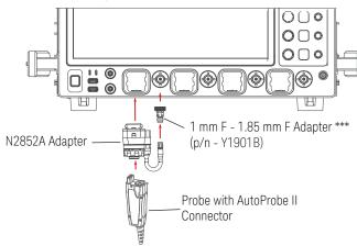
\*\* 1.85 mm F-F adapter is a standard accessory included with 1.85 mm UXR oscilloscope models and not included with N2852A adapter. \*\*\* 1 mm F Ruggedized to 1.85 mm F adapter is an optional UXR oscilloscope accessory and not included with N2852A adapter.
