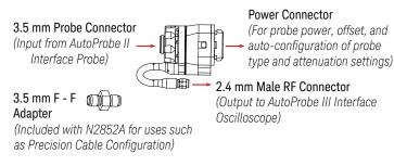
Based on the oscilloscope model, use the appropriate F-F adapter(s) as displayed in the connection diagrams on pages 3 and 4 to connect N2852A to the oscilloscope's input
