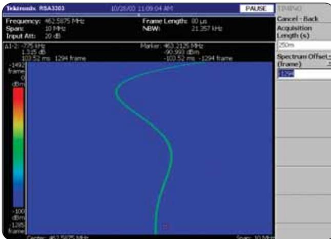
► RSA Series Spectrogram uniquely shows time-varying signal behavior in frequency change/stability, spectrum occupancy, pulsed signal timing, power change and more! The sample on this page shows the frequency settling characteristic of a transmitting device.
