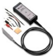
The ZS Series probes provide high impedance and an extensive set of probe tips and ground accessories to handle a wide range of probing scenarios. The high 1 M $\Omega$  input resistance and low 0.9 pF input capacitance mean this probe is ideal for all frequencies. The ZS Series probes provide full system bandwidth for all Teledyne LeCroy oscilloscopes having bandwidths of 1 GHz and lower.
