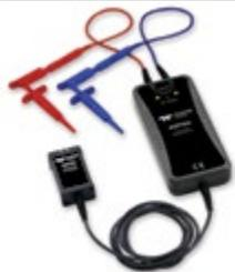
HVD Series high voltage differential probes permit measurements on power electronics circuits with floating voltages without reference to the ground, allowing the oscilloscope to be safely grounded. Excellent CMRR is provided at high frequencies and is combined with low inherent noise, high offset voltage capabilities, and high DC gain accuracy to make them an ideal choice for probing high voltage and floating control signals in single and three-phase power electronics designs.
